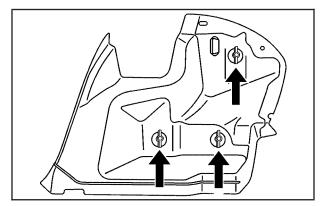
4. Remove the three wing nuts, which hold the taillamp assembly, from inside the vehicle.
